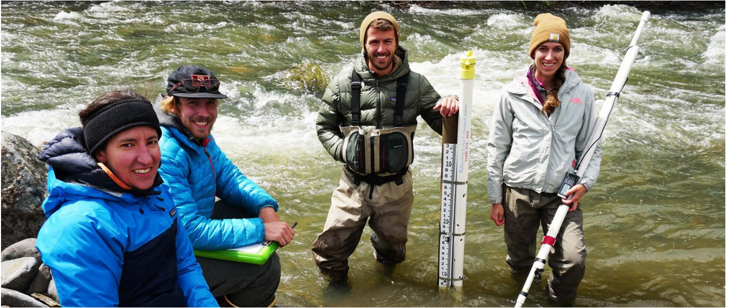
YERC's RiverNET field crew taking measurements on Mill Creek in Paradise Valley to convert stream depth to discharge (flow) for dissemination on RiverNET's web platform. Left to right: Mikaela Howie, Kyle Roberts, Spencer Link, and Morgan Squires.
