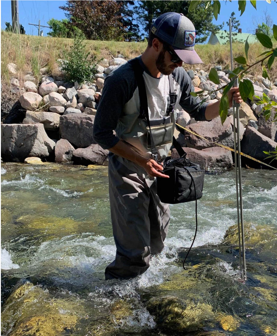
Lead RiverNET Field Technician Spencer Link collects river quantity data along a transect. Photo by Chloe Lo Faro.
